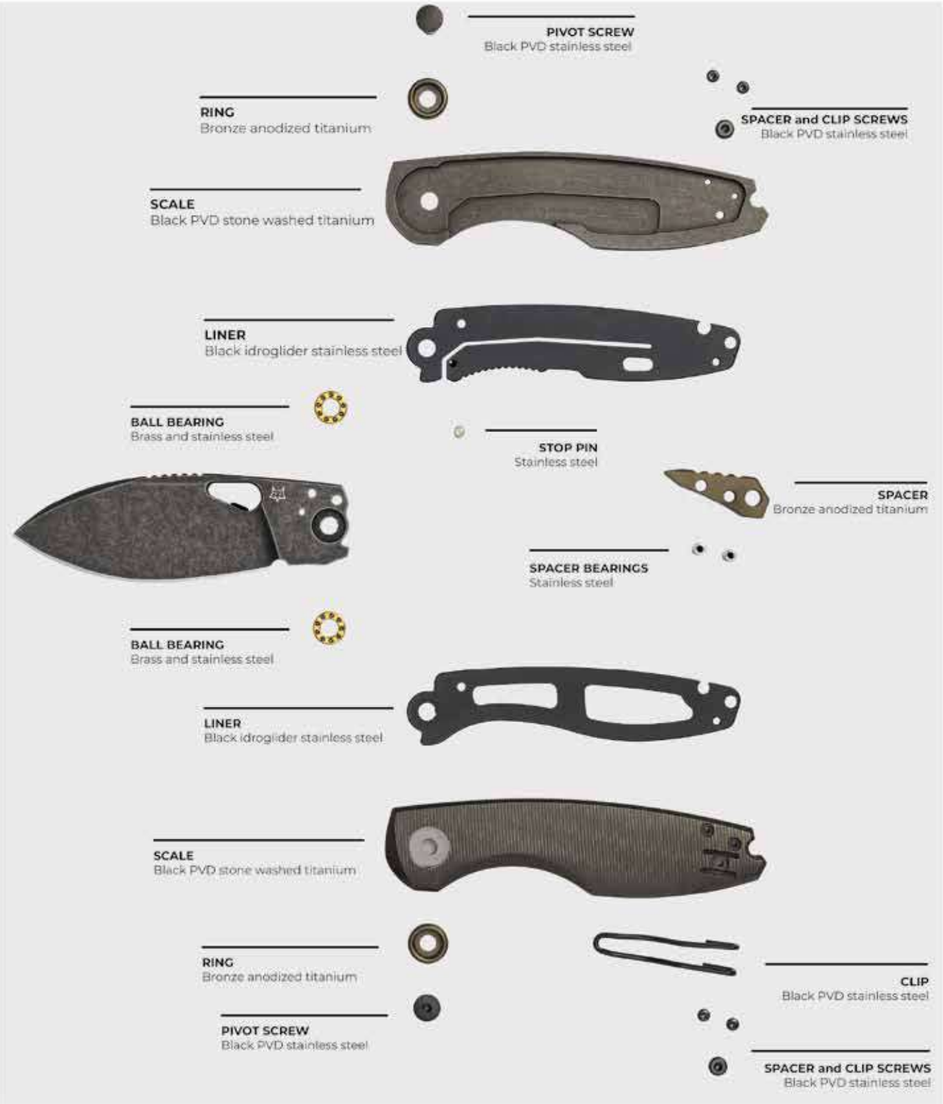
CHILIN FX-530 TIDSW | designed by VOX M39B PVD nero stone washed | Black PVD stone washed M390 Manico titanio PVD nero stone washed | Black PVD stone washed titanium handle
