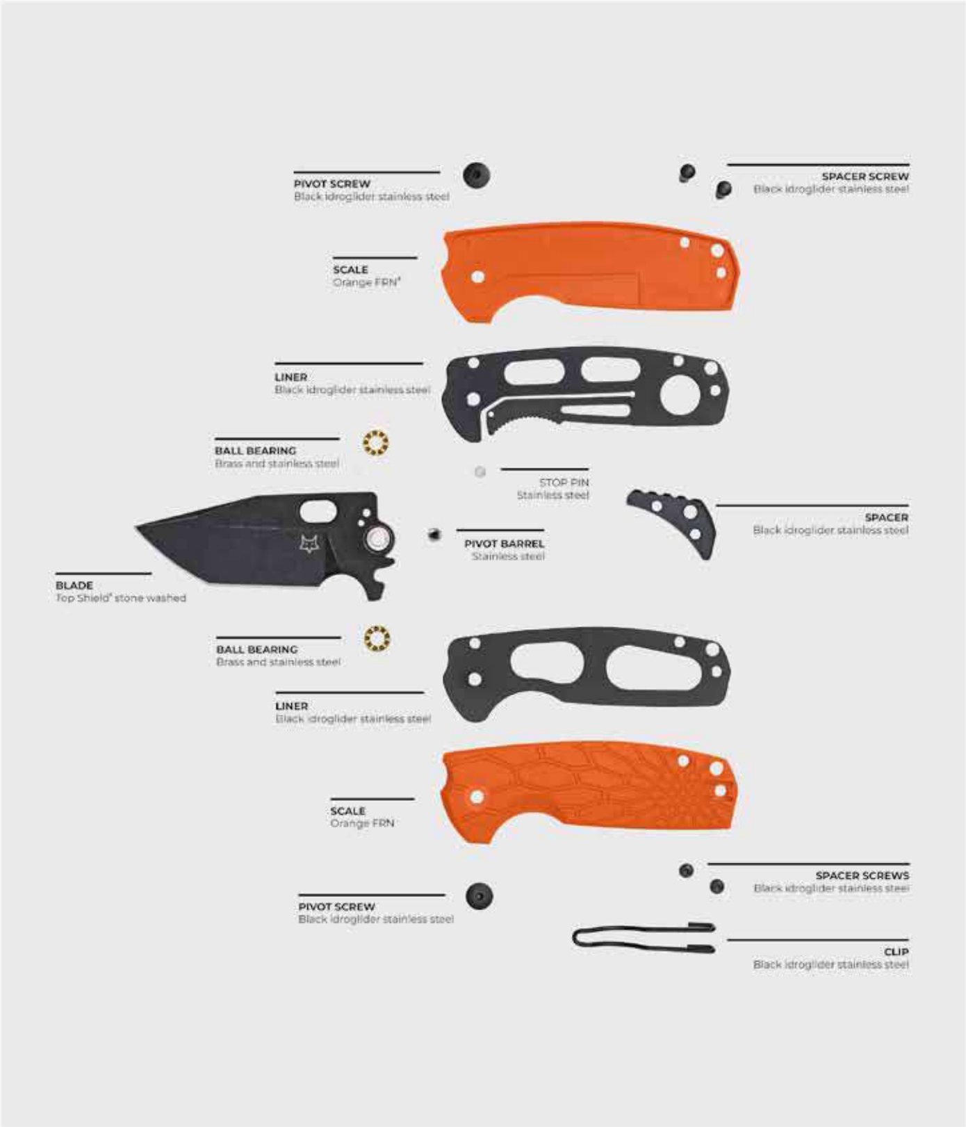
CORE TANTO FX-612 ORB | designed by VOX N690Co black idrogliider stone washed | Black idrogliider stone washed N690Co Manico FRN® arancione | Orange FRN® handle
