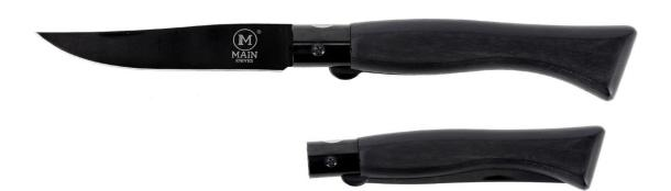
ITEM CODE 10002 STEEL Stainless steel 440 with Black Titanium coating HANDLE Black pressed wood LOCKING liner lock BLADE 87 mm OPEN/CLOSED 203/116 mm WEIGHT 58 g
