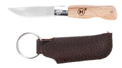
ITEM CODE 6001 STEEL Stainless steel 440 HANDLE Beech wood, leather pouch LOCKING No lock BLADE 45 mm OPEN/CLOSED 100/56 mm WEIGHT 14 g
